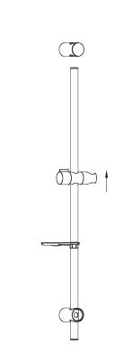
4.Put the stainless steel tube assembly from bottom to top into the upper wall support.
