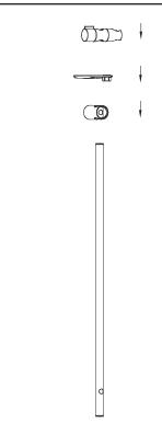
3.Put the down wall support assembly, soap dish and the central part into the stainless steel tube in turn according to the direction shown.
