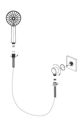
6.Screw the water inlet elbow into the outlet end, ensure the O-ring is to create a watertight seal. Take out the hose, screw one end of the hex nut into the water inlet elbow joint, make sure rubber seal with stainless steel filter exist. Screw the other end into the shower thread joint, make sure rubber seal rings and flow restrictor installed.
