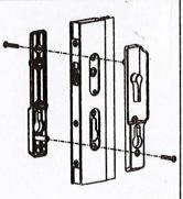
Step 4: Insert the cylinder into lock-body and the cam of cylinder face towards the front end of the door. Secure the cylinder with 31.7mm countersunk screw provided, prior to tighten the screw of cylinder, please check the cylinder and lock-body function with key.
