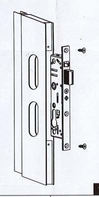
Ensure the cylinder cam is inside the cylinder & the locking bolt is fully extended, then insert the cylinder and fasten with the screw provided.
