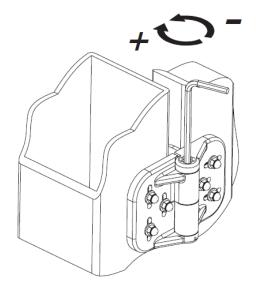
MAINTENANCE: The hinge should be inspected annually, or more frequently if the gate is used often. Spring tension adjustments should be made as needed.
